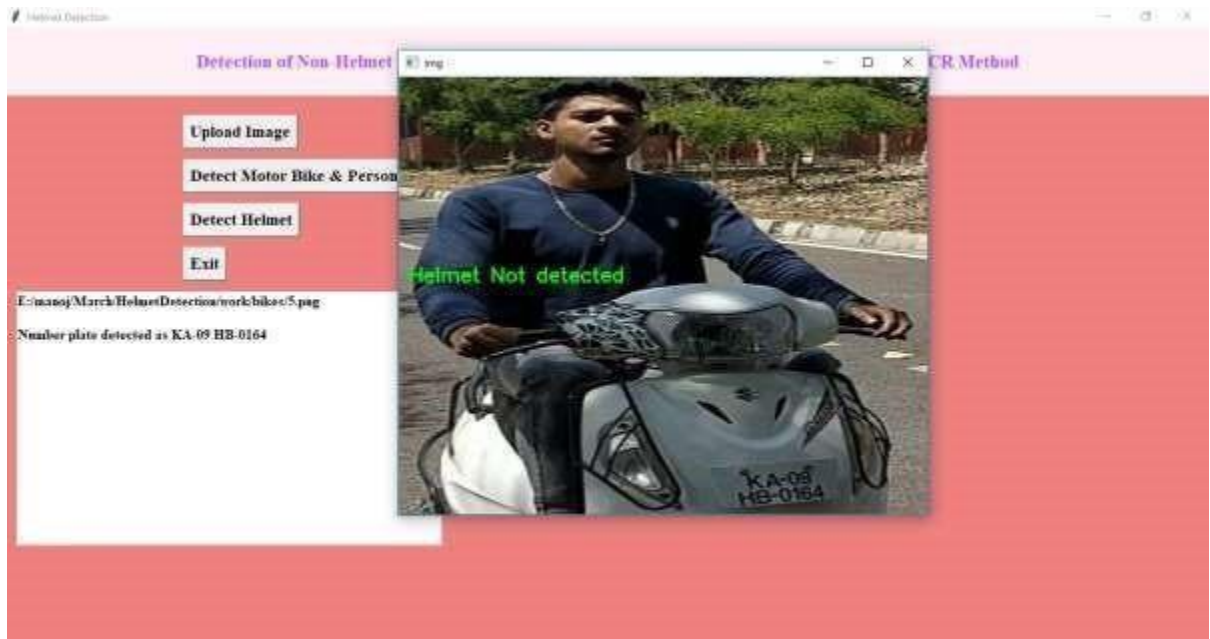
Fig. 6 Screen page displaying the vehicle number when no helmet is detected
